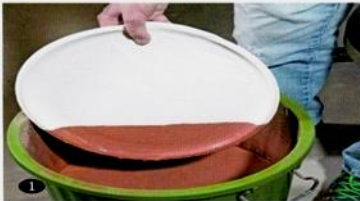
The glaze should be thoroughly mixed to prevent denser and heavier materials from settling to the bottom.
