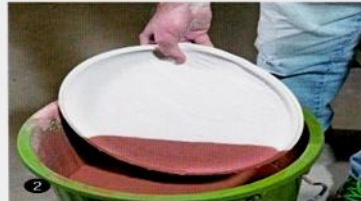
The plate is slowly dipped into the glaze, distributing an even coating. Larger forms require greater care, as the weight of the glaze suspended in water can cause cracking due to overstraining the bisque pottery.
