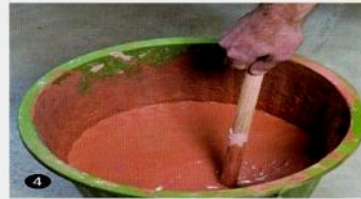
Some glazes, depending on the density of their raw materials, require frequent stirring to keep the glaze in suspension.
