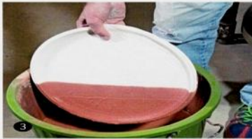
Hold the plate in a vertical position to prevent the water weight contained in the glaze from cracking the bisque.
