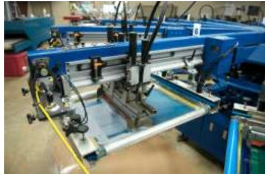
Gambar 2.21 Contoh mesin rotari cetak saring (*Rotary Silk Screen Printing Machine*)
