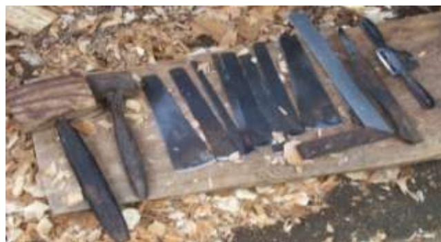
Gambar no. 15 Palu kayu, Pahat, Siku, Pemutik, Serut Yuyu Foto : I Made Berata
